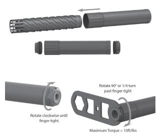
Assemble the front cap finger tight first, then thread the Mount Base into the housing until finger tight. Using the provided RAD 22 Wrench or a 3/4" socket, tighten the Mount Base and additional 90 degrees or 1/4 turn past finger tight.
