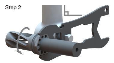
Thread the QD muzzle device directly onto the barrel of the host firearm. Using a HUXWRX QD wrench with torque wrench, index the hex flats on the muzzle device and torque it to approximately 33ft-lbf (45 Nm).
