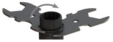
Affix a VENTUM wrench horizontally in a vice and index it onto the wrench flats at the base of the housing. Use an additional VENTUM wrench, as shown, or 15/8" socket on the HUB-QD Adapter flats and torque to 25 ft-lbf (34 Nm).
