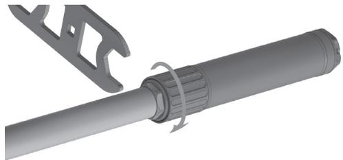
Rotate the RAD 22 suppressor counter-clockwise to unthread it from the host firearm. If needed, the provided RAD 22 Wrench can be used to detach the Mount Base from the host barrel.
