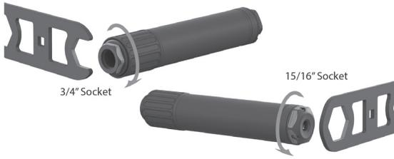
To unthread the Mount Base, use the RAD 22 Wrench, 3/4" socket, or adjustable wrench.
