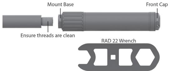
Ensure all mounting surfaces and threads are clean before installation. Ensure the RAD 22 Front Cap and Mount Base components are firmly tightened before mounting to the host firearm.
