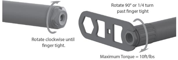
Assemble the front cap finger tight first, then thread the Mount Base into the housing until finger tight. Using the provided RAD 22 Wrench or a 3/4" socket, tighten the Mount Base and additional 90 degrees or 1/4 turn past finger tight.
