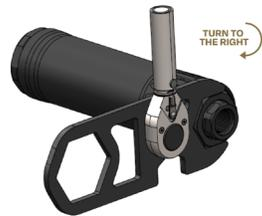
TORQUE PISTON BASE OR DIRECT THREAD ADAPTER TO 100 LBF-IN (115 KGF-CM)
