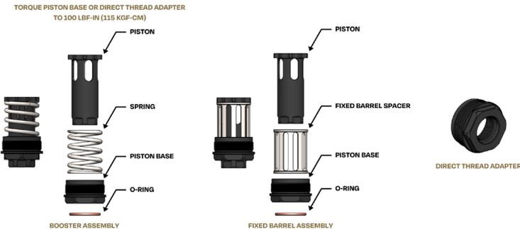
1. The Booster Assembly comes preassembled and greased in the RAD 9 & 45. The Booster Assembly with Spring is necessary to function on weapon systems where the barrel reciprocates to cycle. Use high temperature grease on the Piston, Spring, and O-ring before each session of use.
